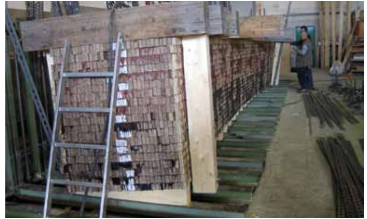
Tests showed that Accoya can be glued just as well as conventional glued-laminated timber when using the specific resorcinol resin.
